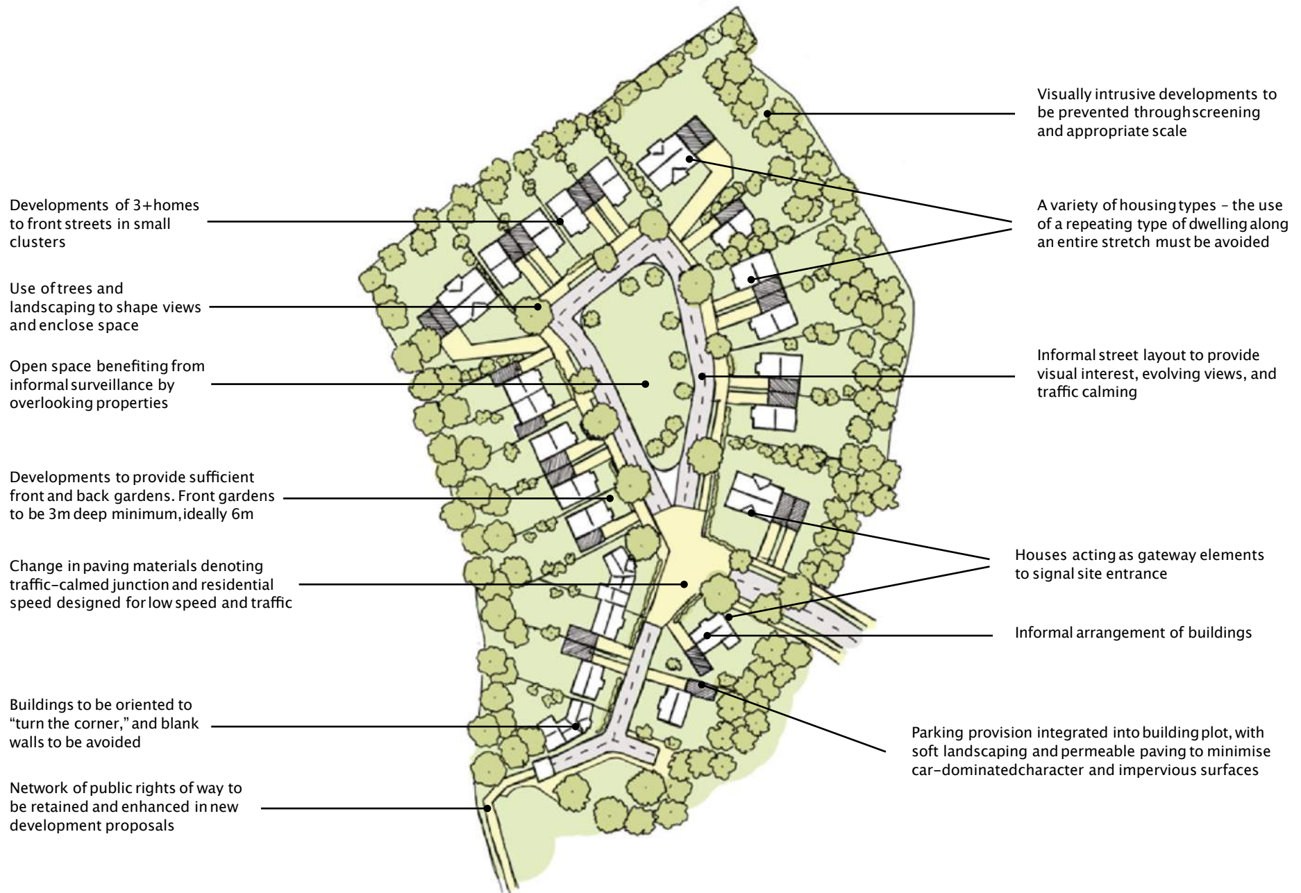
Figure 19: Illustrative plan for a small development highlighting many of the elements of the Sarratt code where they relate to the pattern and layout of buildings.
